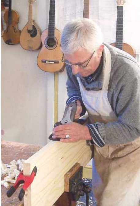
▲ Pic.1 The edges of the shelving boards are planed true
